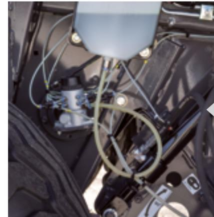
Automatic chain lubrication with individual adjustment for each chain guarantees sufficient oil supply, reduces maintenance time and extends chain service life. For added durability the highest quality chains are used throughout the baler.
