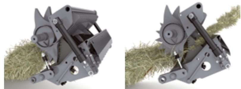
The patented protection system prevents peak loads from turning into blockages by gentle lowering of the floor which is suspended on rubber blocks or steel springs, depending on the model.
