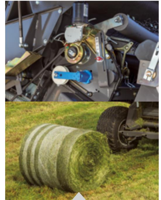
The optional Variotwin twine system offers simple and economical bale tying. The unique Variable Speed Control allows for additional twine revolutions on the bale edges, securing bale ends and increasing overall tying speed, which is particularly beneficial when baling light crops.
