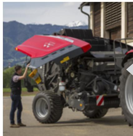
Full width side doors provide easy access for maintenance. The smooth surface design prevents dust accumulation beneath the panels while secure locking prevents unintended opening and potential damage.
