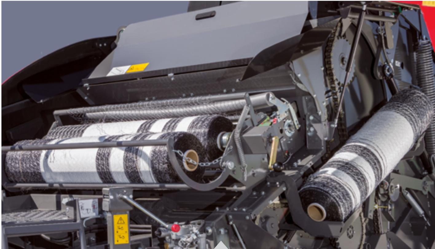
The **Easy Loading System (ELS)** allows one spare roll to be carried on the baler, allowing for roll replacement to be made in a matter of minutes. In addition to ELS most specifications feature storage for an additional, third net roll on the left hand side of the baler, increasing effective time in the field even further.
