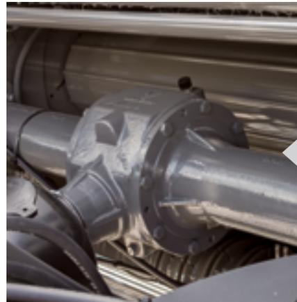
The Powersplit gearbox equally divides and transfers power to drive the rotor unit on one side and the roller drives on the other, reducing the overall power requirements by simplifying the drivelines. This results in a more efficient baler which uses less fuel.
