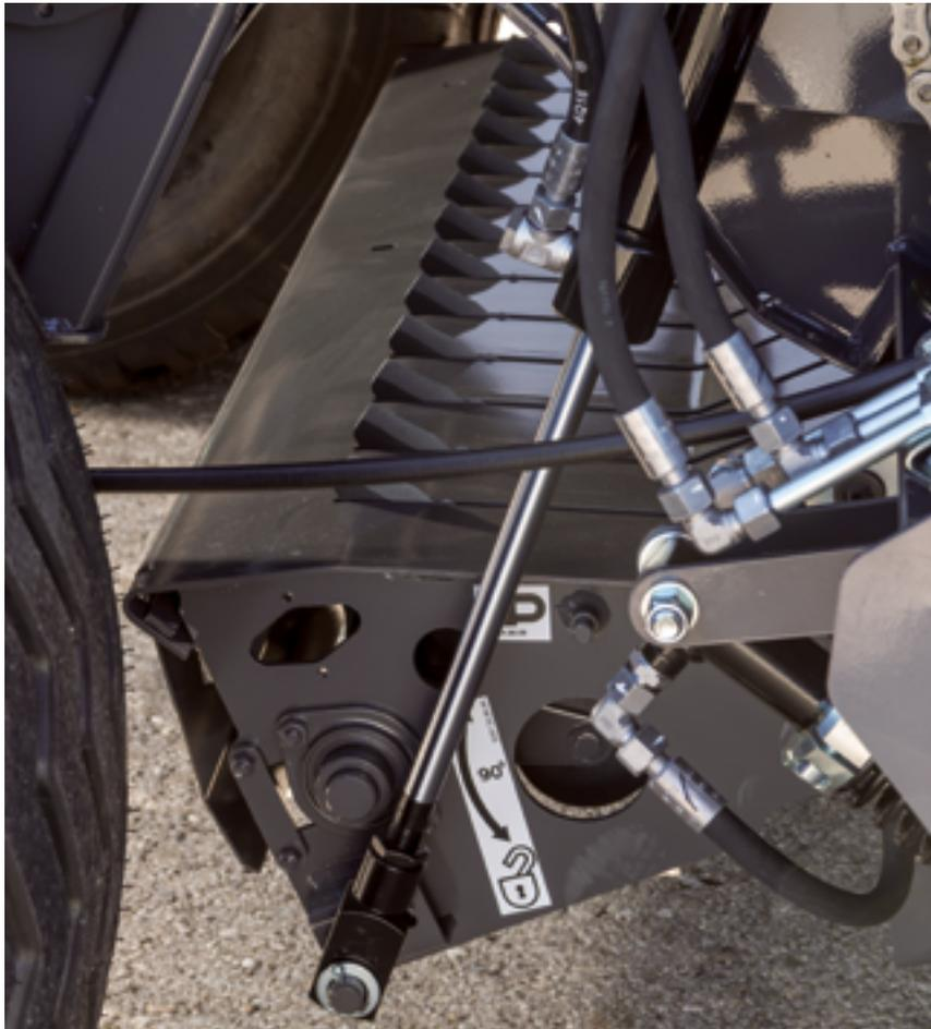
The first stage of Hydroflexcontrol allows movement of the front part of the feed chamber floor and will automatically prevent up to 80% of potential blockages and will keep you going without unnecessary downtime.
