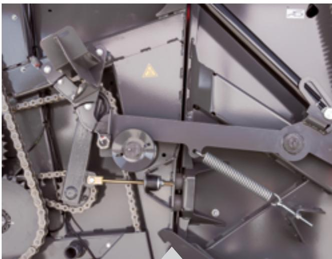
Mechanical tail-gate locking device; simple, fast and efficient, resulting in uniform bale diameter, high density bales and lower power consumption.
