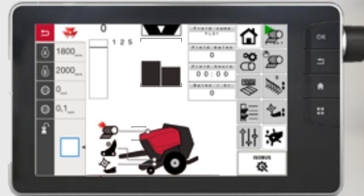
If a tractor is fitted with ISOBUS control, it is also possible to use the tractor's monitor to view all the key information about the tractor and the baler in one place.
