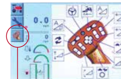
A handle configuration icon in the FieldMax Monitor will always be visible, so you can view and/or change handle settings with a single button.
