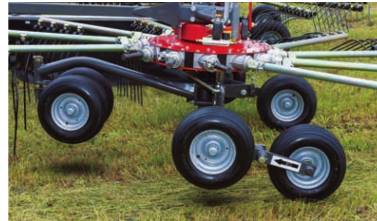
Patented, fully cardanic rotor suspension
