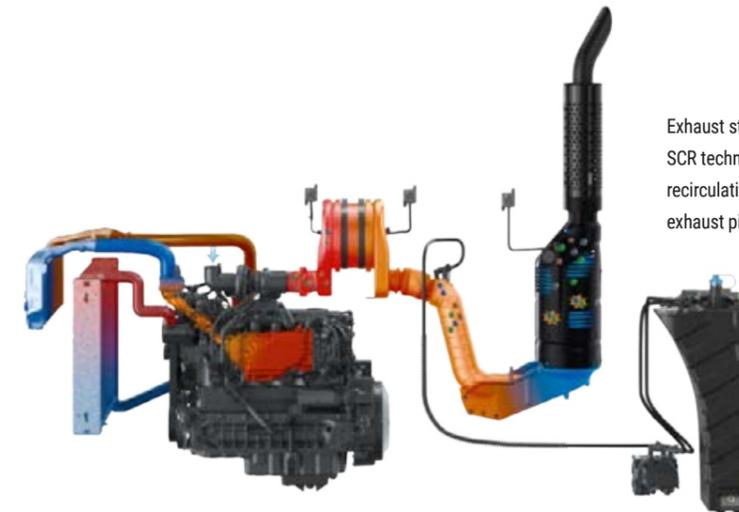
Exhaust stage V is met thanks to the external exhaust gas recirculation, SCR technology and diesel particulate filters. The external exhaust gas recirculation reduces the nitrogen oxides (NO<sub>x</sub>) even before reaching the exhaust pipe, so that AdBlue is used particularly sparingly.
