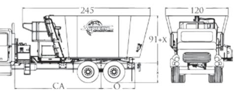
Height of truck frame to top of tub. Add to truck frame height for overall height.
