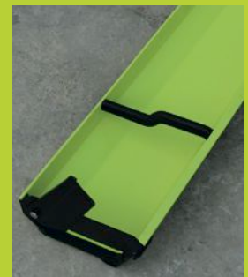
Calibration test's tray with emptying shutter.
