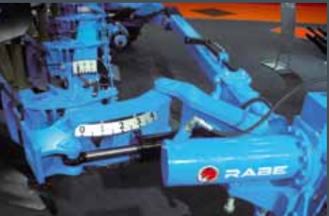
Robust double joint for setting the first furrow width or the on-land version. While ploughing "in the furrow" it is possible to 'slip' the first furrow (very useful in difficult conditions).
