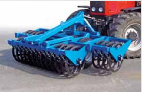
Combination of casting ring packer and packer for an even consolidation across the width of the machine.
