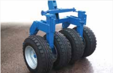
Combination of casting ring packer and packer for an even consolidation across the width of the machine.
