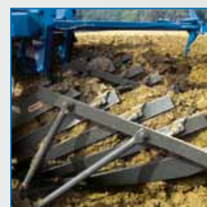
Clod breaker for additional soil crumbling right on the moldboard.
