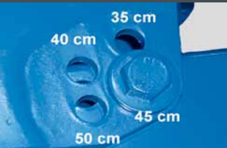
Bracket with four-step working width adjustment (35, 40, 45 and 50 cm).
