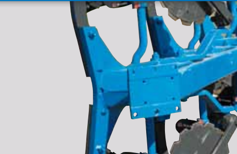
Simple expandability of the plough by an extra rear furrow.
