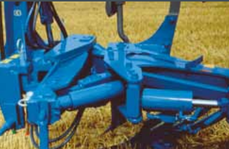
No moving of the bodies during turnover, because of the alignment cylinder. This reduces the turning points in motion for less wear. Standard from up 5 - furrows.
