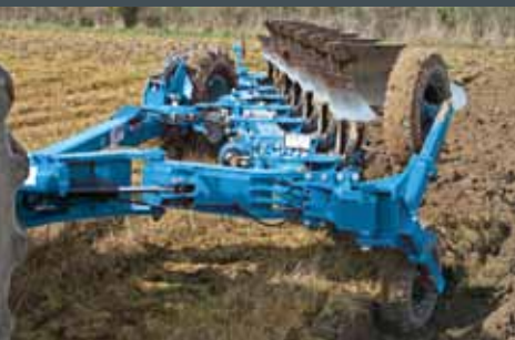
The Kormoran in on-land version can either plough on-land or in-the-furrow.
