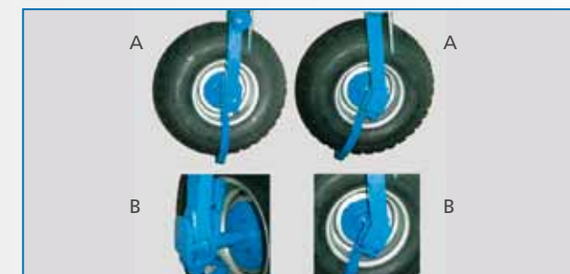
Damper (A) for gentle rotation and strake (B) to stop the wheel going forward.
