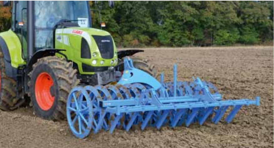
Front press with cast rings for a good consolidation and fragmentation, ring diameter 70 cm and 90 cm, also with leading tines or blades available.
