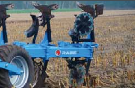
Simple expandability of the plough with an additional rear furrow. (necessary if the wheel track is to be ploughed).
