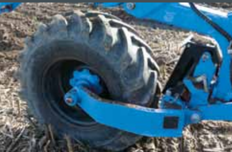
Big dimensioned wheel provides high directional stability, directs with the turning.
