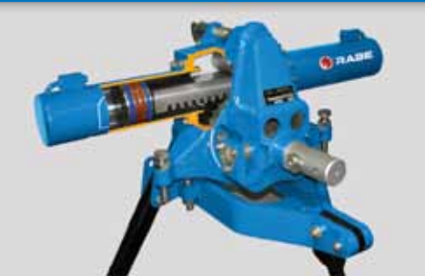
Controlled turnover without top dead center by the rack and pinion.
