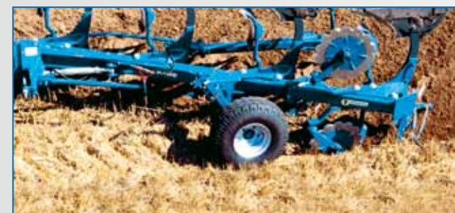
Lateral wheel for uniform depth control with damper and strake can be mounted front or rear. (For Albatros / Super Albatros)
