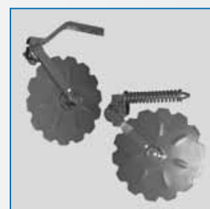
Disc coultter (Ø 50 cm), optionally with suspension for stony grounds.
