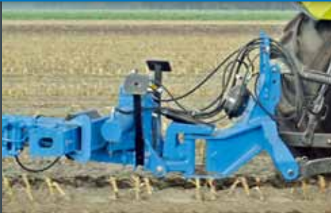
Controlled turnover without top dead center by the rack and pinion. Middle axle can be "steered".
