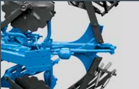
Hydro Avant auto reset or simple shear bolts for stone protection.
