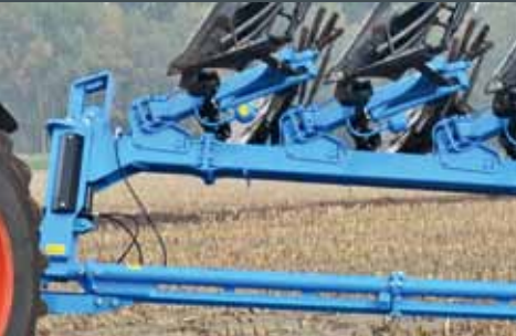
Easy expandability of the plough with an additional middle furrow. Allows the possibility of future expansion up to 9 furrows (8- furrow with hydraulic auto reset).
