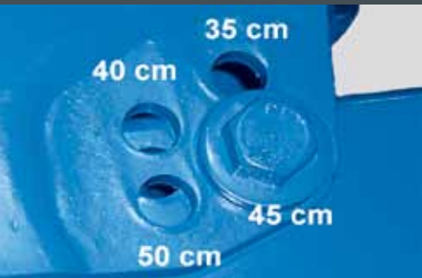
Furrow with four-step working width adjustment (35, 40, 45 and 50 cm).
