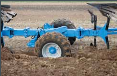
Plow frame with joint to follow ground shapes. Automatically locking in excavation and transport position.
