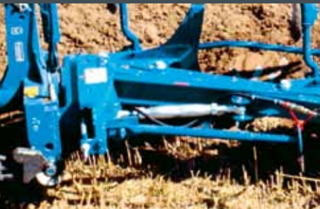
Change of working width does not require any adjustment of first furrow and true line.
