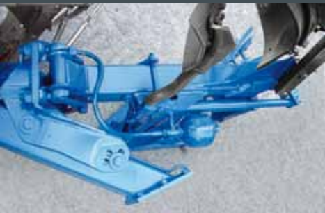
Proven Rabe system: hydro-avant hydraulic stone protection.
