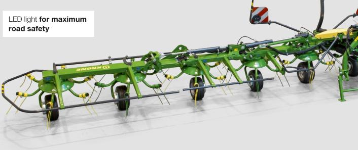
Gauge wheels run close to the tines providing **exact tine control and optimum forage quality**
