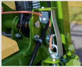
**Manual border spreading control** The border spreading facility on the Vendro 470 to 790 models is operated on this cable from the cab.
