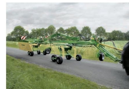
Swadro 710/26 T Work width: 6.20 m (2 rotors of 3.40 m each)
