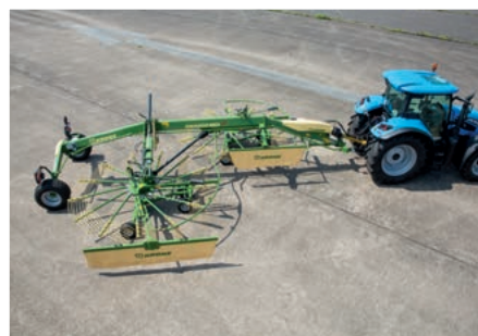
Swadro TS 740 Twin Work width: 7.40 m (2 rotors of 4.10 m each)
