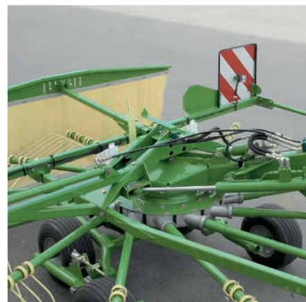
Shifting the rear rotors left/right
