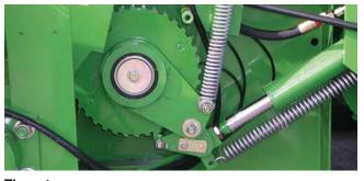
**The rotor reverser** The cut-and-feed rotors can be reversed manually or hydraulically as an option.
