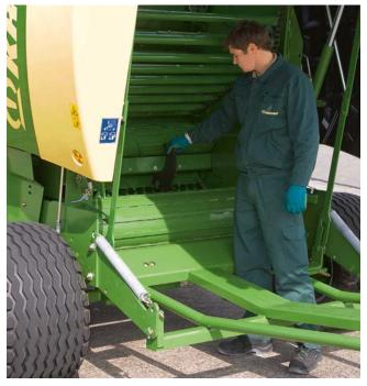
**Changing the blades** Unlock the knives and remove them from above for grinding or replacement. No tools required.
