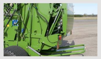
**High-density and well-shaped bales** On the variable chamber model, two hydraulic rams, one on either side of the rear door, exert the full baling pressure at the rear of the baling chamber.
