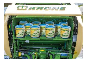
**The storage compartment** The large storage compartment holds up to 11 balls of twine. Hoops hold the rolls in place for smooth uncoiling.
