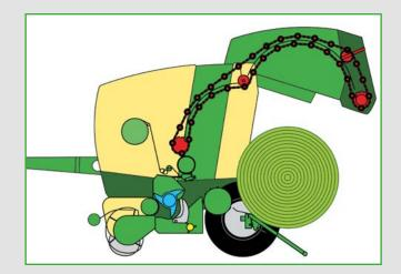
and so the baling cycle finishes earlier as well. The elevator also creates a firmer core and packs more weight and density into each bale, which translates into higher quality silage and better exploitation of truck capacities.
