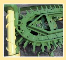
Automatic tensioning extends the service life: The **Collector** is tensioned automatically by means of a compression spring. The spring pushes the idler wheel outwards, so that optimal tension is always ensured on the Collector.
