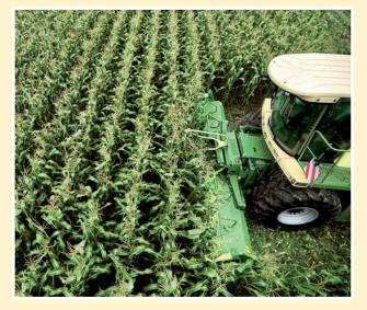
EasyCollect 6000 FP operates independently of rows, which has many advantages: The harvester can travel transverse of the rows, there is no dependence on row spacing – tight row spacing or a 90 cm (35") spacing is not a issue. This helps when harvesting down crop as the crop can be approached in any direction. Builtin is an adjustable headstock which adapts the head to the forager to achieve the correct cutting angle.
