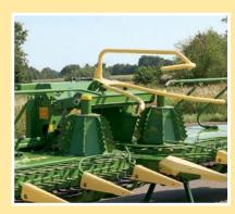
Adjustable bullhorns: The bullhorns ensure a perfect feed of the plant into the feed rolls. It can be simply adjusted via a pin so it can adjust for every crop condition.
