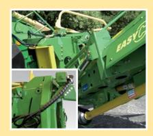
Fast attachment and removal: The EasyCollect heads have several adapter frames specially designed to fit the forage harvester regardless of make and model. KRONE offers the correct frame to fit. Also the heads are very easy to mount just a few minutes and the machine is ready for chopping.
