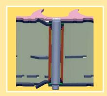
Precision cutting: The stalks are cut in a simple scissor-type manner. The continuous rotation of cutting knives on the Collector pulls the plant against a serrated stationary knife for a quick and clean cut. The easily replaceable knives are coated with tungsten carbide and are self-sharpening, once again a maintenance friendly system.
