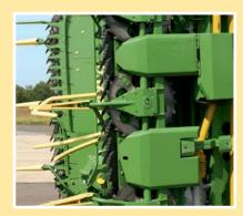
Extra wide skids protect: The EasyCollect 6000 FP has extra wide skids as a standard feature. They can be fully adjusted to guarantee you get your desired cutting height with a constant stubble height.
