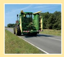
Safe on the road: The tips of the stalk lifters are covered by the front guards when transported on public roads. With the integrated lights and indicators, travel is absolutely safe even at night – safely out in front.
