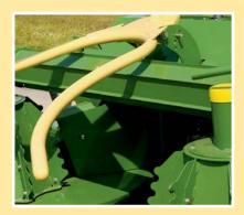
Stalks first: The deflection roller presses the plant bundle forward so that the stalks are guaranteed they are being fed "Feet First". The "Rolling Change-Over" guarantees a continuous and loss-free crop flow.
