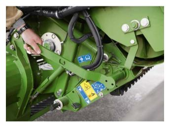
**Standard feature: manual blade group control** The standard manual control is a long lever that takes little effort to operate. This way you can quickly adjust the number of blades to varying conditions and customer needs.
