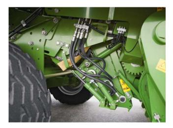
**Optional feature: hydraulic blade group control** The hydraulic blade group control system is an option and the system is operated from the convenience of the cab, saving valuable time.
