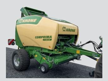
build and design. It can unload bales of different diameters and compacts from the outside to the inside; with larger bale diameters, it leaves only a very small soft core. Thus, it achieves high bale weights.
