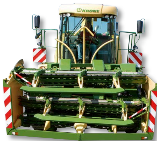
Compact transport position: The triple-fold EasyCollect header
