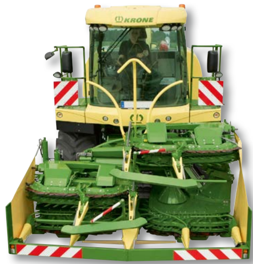
Compact transport width – the triple-fold EasyCollect corn head
