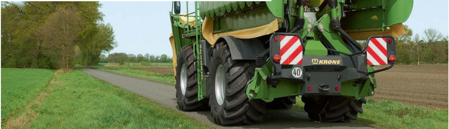
The hydraulic transmission on KRONE BiG M 500 steers through tight turns and provides modulated control when inching up in confined space. The four-wheel drive is permanently engaged. In the field the machine operates at a max. 20 km/hr (12.5 mph) and on roads at a max. 40 km/hr (25 mph). You can split the circuit as required to have each axle supplied with oil by a separate pump, offering maximum traction in difficult terrain.
