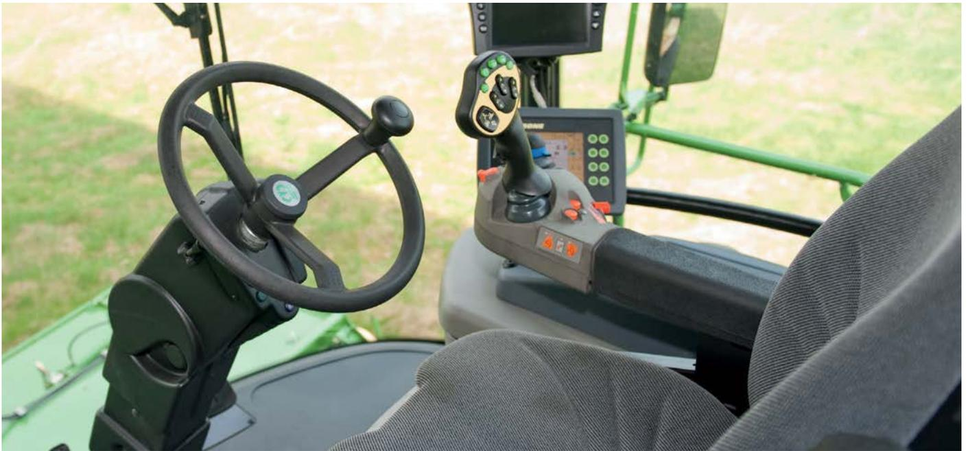
BiG M 500 features four-wheel steering as standard specification. The operator can choose between various modes.
