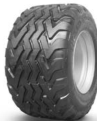
Radial ply tyres 620/40 R 22.5 TL Width: 610 mm Ø: 1,080 mm
