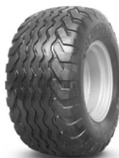
Cross ply tyres 500/55 R 20 TL Width: 505 mm Ø: 1,060 mm
