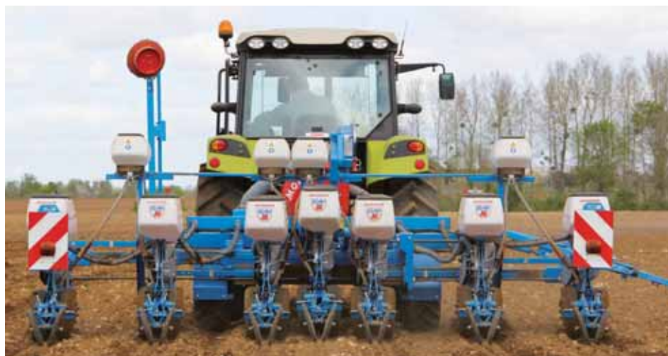
The mixed 6/7 row Extend version offers spacings of 75 and 80 cm in 6 rows and of 55 and 60 cm in 7 rows. It is thus possible to change very quickly with no disassembly, from 6 rows maize to 7 rows sunflower/rapeseed.
