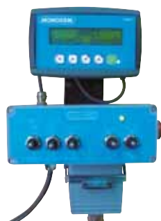
The electric distributors enable to control all the functions of the planter with just one double acting distributor. An automatic control at the field end lifts the folding parts and the rows markers in order to maneuver safely.
