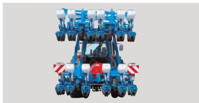
The central part of the frame is made up of a double telescopic frame, the wings are telescopic and folding for a transport width of 3m (depending on the equipment).
