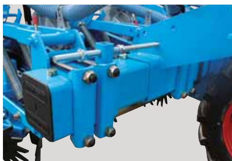
The stop parts on the telescopic system enable an adjustment perfectly suited to the required inter row spacing and folding that is suited to the equipment of the planter.
