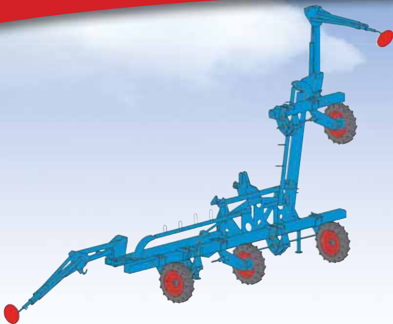
12-row Double bar folding planter (45 cm inter row spacing)
