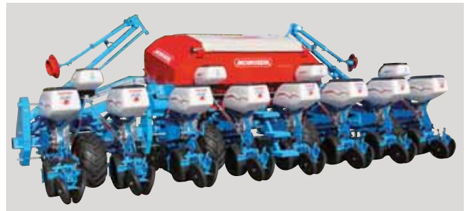
8-row TFC floating frame (75 cm inter row spacing)
