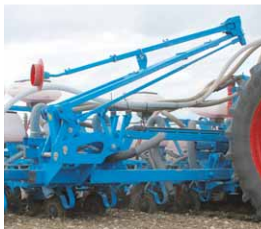
The compact folding row markers enable marking at the wheel or at the centre and take up little space when in transport. They are also equipped with a safety system.
