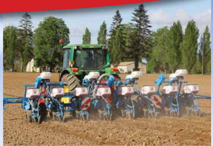
8-row Double bar folding planter (80 cm inter row spacing)
