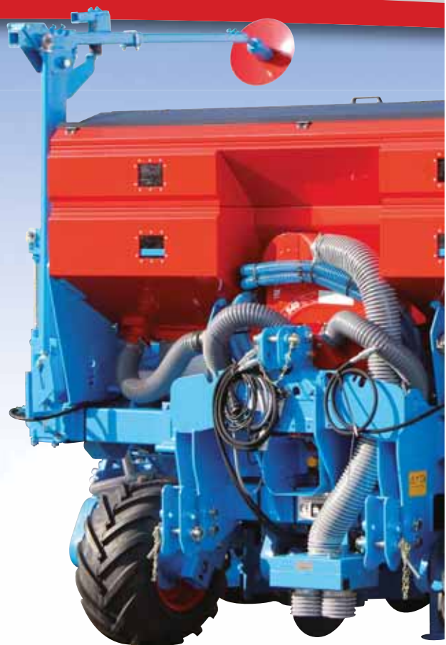
6-row Monoblock2 Comfort planter with fertilizer 1030L and Combined Microsem (75 cm inter row spacing)
