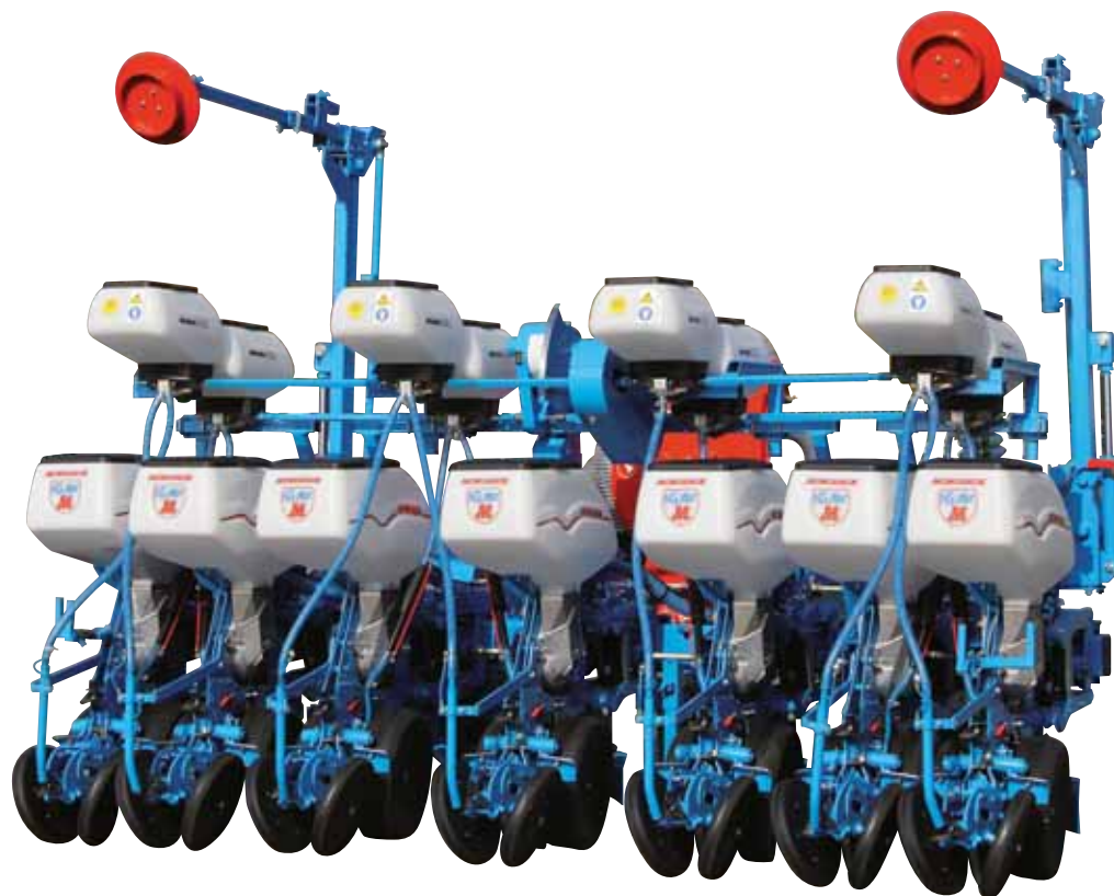
7-row Monoblock2 Comfort with Combined Microsem (60 cm inter row spacing)
