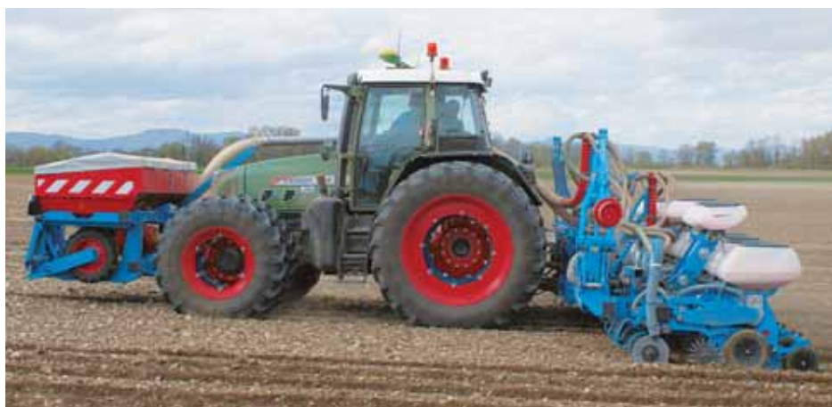
The CRT frame can be equipped with standard fertilizers (4 x 270 L) or the equipment for the front-mounted Standard or DUO fertilizer. In this configuration, the planter has 2 distribution heads (assembly according to inter row and equipment).
