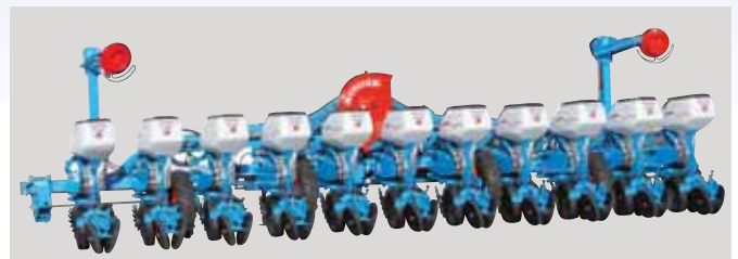
11-row Double bar folding planter (60 cm inter row spacing)
