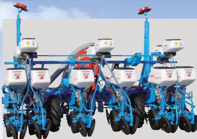
6-row Monoblock 260 single telescopic planter with Combined Microsem (75 cm inter row spacing)
